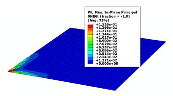
Figure 4: Cracking of isolated simply supported slab.
