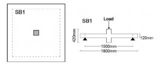
Figure 1: Schematic drawing of the isolated interior slab-column connection SB1.
